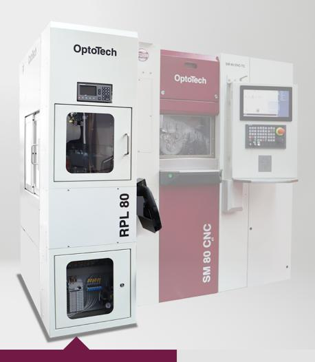
The RPL 80 is the high performance robot solution from OptoTech, that allows automatic loading and unloading of the SM 80 CNC-TC generator, the SPK 80 CNC polisher as well as the OWI 60 HP Invers-A interferometer. The RPL 80 can handle single surfaces (up to  $\emptyset$ 80mm) as well as lenses on cementing pieces.
