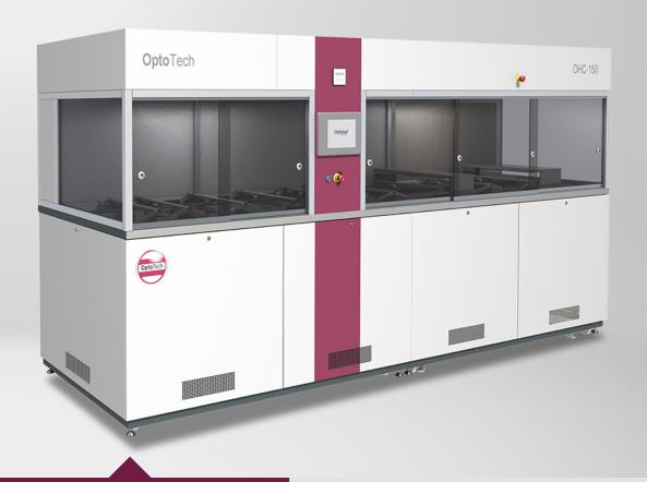
The OptoTech Hard Coating System (OHC) combine cleaning with ultrasonic and thermal cure dip coating for ophthalmic lenses. The OHC hardcoating systems are characterized by the product quality for which OptoTech is known, ease of use, and exceptional reliability in the daily production operation. Our hardcoating systems use well proven technologies to deliver lens surfaces that are pristine and contamination-free.
