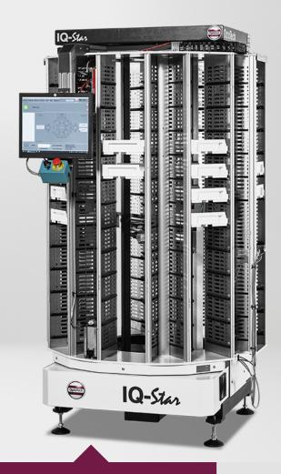
space saving and intelligent LAB automation, which links the storage and distribution of job trays in an intelligent manner.
