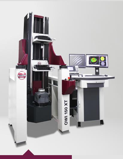
High precision Fizeau workshop interferometer OWI 150 XT 1500 for testing of spherical and aspherical surfaces. High precision kinematics and a working range up to Ø 150 mm make this measuring machine an indispensable tool for the production of highend optics.
