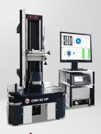
The compact Fizeau workshop interferometers OWI 60 HP and OWI 60 HP Invers are ideal tools for measuring of optical components. Several options allow the adaptation of these measuring devices to individual measuring tasks.
