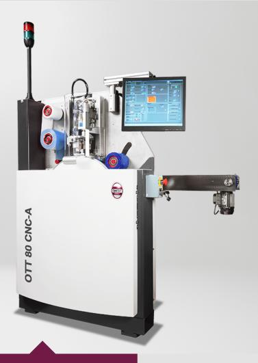
The ultimate lens protection for semi-finished blanks. OTT 80 CNC A is a fully automatic system for applying a protective film (tape) and the fastest on the market. It is the ideal and flexible taper for small, midsize and big laboratories.
